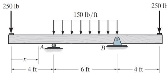
**(c)** Draw Shear force and Bending Moment Diagram for Q.2 (b) **07**
