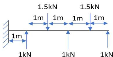
**(b)** Determine Support Reactions for beam given below.
